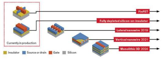
**New Geometry:** Eventually, miniaturization may be supplanted by monolithic 3D integration, which would build layers of devices, such as the planar transistors shown here, atop one another, connected by dense wiring. Older technologies will continue to be used.
